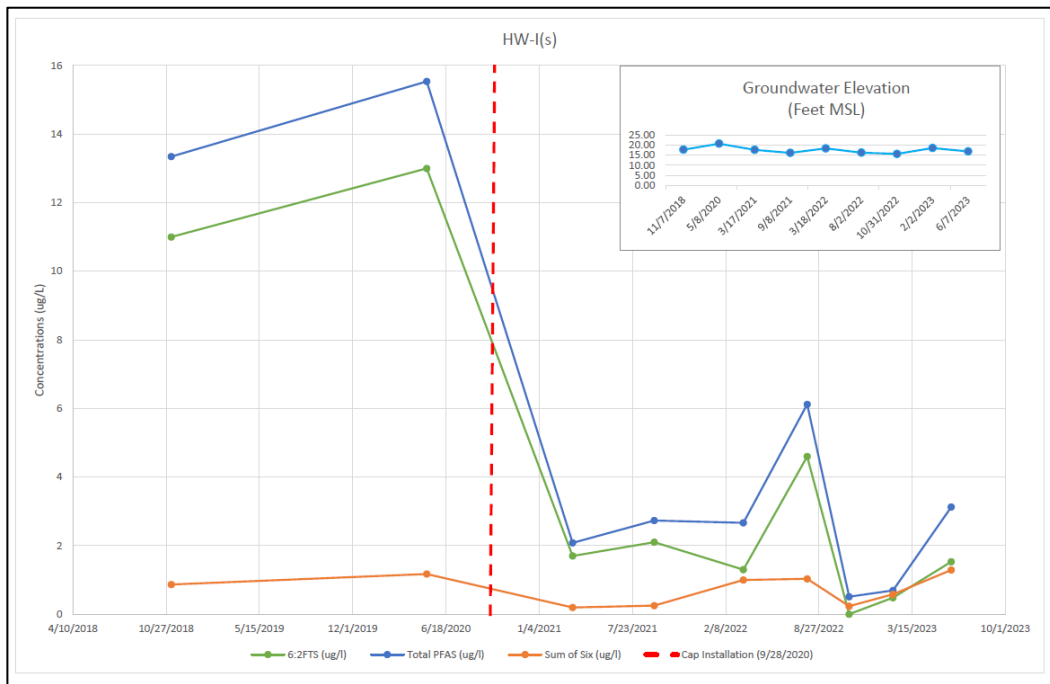
Figure 3 Graphic From Airport's Phase IV Report concluding significant PFAS reduction from the Cap Installation focusing on the non-regulated 6:2 FTS
